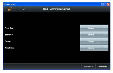
8. For each lock on the Permissions detail page, indicate if the user has permission to access the lock (Enabled) or not (Disabled). Use the buttons at the bottom of the screen to enable or disable all the locks for this user.
