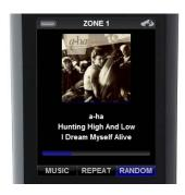
**Button Display**: The thin line at the bottom of the touchscreen is actually three buttons that are contextual and become accessible when you press the corresponding arrow (▲) button below the touchscreen. For example, Random was toggled on by pressing the right-most arrow (▲) button.
