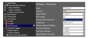
4. Either right-click on the desired IR code and Add an Event Map for IR Code Begin Receive or go to the Event Mapper tab and add a new event with the trigger: System Family: Input/Output, the IR Device: IR Code, and IR Code Begin Receive.
