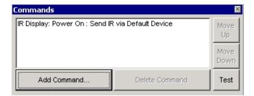
**Note:** If the Commands window does not have a command populated, it is most likely because the command name does not match the Universal Function of the command. Commands can be added manually by clicking the **Add Command** button.
