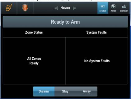
5. Try to Arm the system. Click **Away**, then click **1**, **2**, **3**, **4** and **Enter** in order (this is the default security code for the Virtual Security device). *After a short delay, the display will show* **Armed**.
