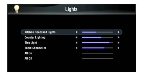
Remote Function: For the Lighting section of the OSD, the standard cursor controls are used for navigation. Select a specific light by highlighting it with the cursor to make it active. When selected, the arrow keys can be used to raise/lower lights. For toggle controls, the OK button will toggle between On and Off states. If the default media zone is active, hard buttons will still pass to the default media zone.
