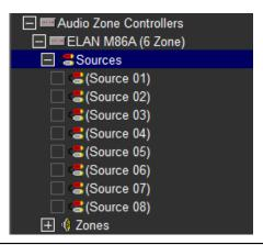
**Note:** The names shown for sources should match the input names printed on the back of the zone controller
