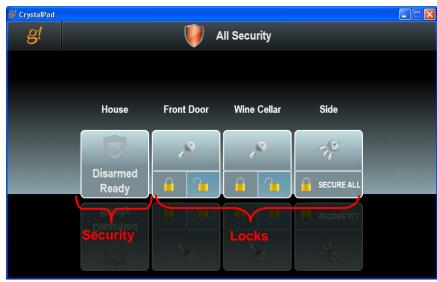
3. Click the closed padlock symbol on the **Front Door** to secure the door. *The* system will indicate that it is working, and then the icon will turn blue.
