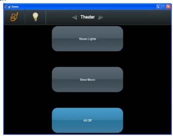
3. Click the light bulb to return to the available lighting interfaces then click the Custom Tab. You should see the Theater Keypad on the left, the toggle controls on the upper right, and the dimmer controls on the lower right. Click the buttons on the Theater Keypad and verify that the controls associated with each button move to their intended position.
