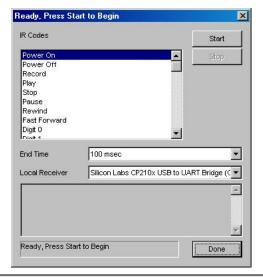
**Note:** By default, the **End Time** is set to **100 msec**. This value can be reduced to help capture codes from remotes with shorter pauses between repeated commands.
