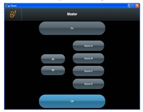
**Note:** The Configurator adds Viewer interface pages for each keypad by default. Note that individual loads (switches and dimmers) don't automatically display in the interface.
