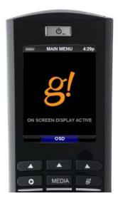
When in OSD mode, the HR2 hard buttons will mimic the g! remote buttons. The HR2 has two additional hard buttons: Now Playing ▶ and g!, which are not present on the g! remote; so when the **Now Playing** button is pressed, it will jump the OSD to the **Now Playing** screen. When the **g!** button is pressed, it will jump to the OSD main menu.
