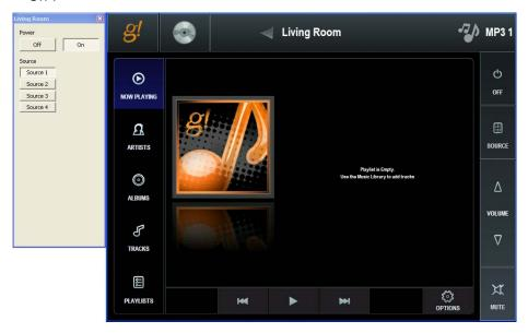
8. Click the **Source** button on the right, select the **AM/FM Tuner** source and click the **Keypad** button. The AM/FM Tuner interface displays, the Living Room Virtual Zone changes to "Source 3", and the source indicator (icon and name) to the right of the Living Room heading changes.
